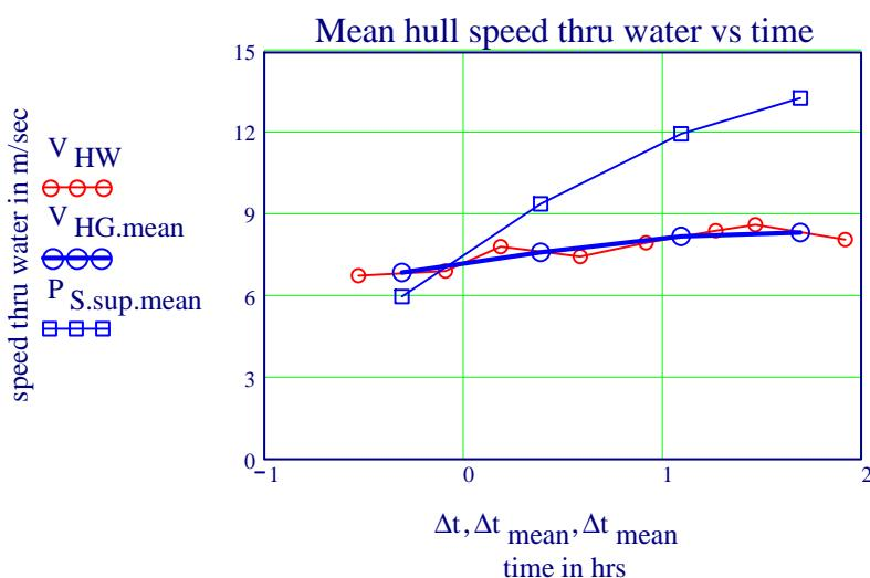
In the present case the mean speed over ground happens to be equal to the speed over ground at the mean time between the two corresponding runs.
