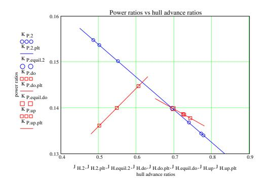
According to these results the nominal no wind and waves powering performance at the smaller trim differs from that at the larger trim even in the non-ventilating condition. One of the reasons may be the surface effect due the very small nominal submergence of the propeller.
