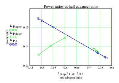
Evidently the propeller is ventilated at the up-wind condition. Thus the global evaluation is non-sensensical, particularly with 'corrected' values!
